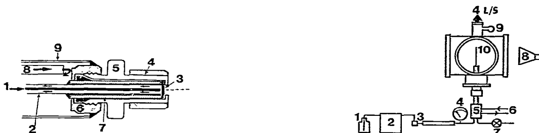
Fig. 3. Schematic cut section of the DLI interface end. 1 = Input tube (0.15 mm O.D. \times 0.1 mm I.D.); 2 = output tube (1.56 mm O.D. \times 1 mm I.D.); 3 = diaphragm (3 mm O.D., pinhole 1-3 \mu\text{m} ); 4 = spacer making seal against ion source block; 5 = modified Swagelock (Cleveland, OH, U.S.A.) reducer (SS-200-R-4); 6 = Swagelock nut (SS-202-1); 7 = holder tube (3.17 mm O.D. \times 1.56 mm I.D.); 8 = temperature-regulating water input; 9 = interface end shaft.
